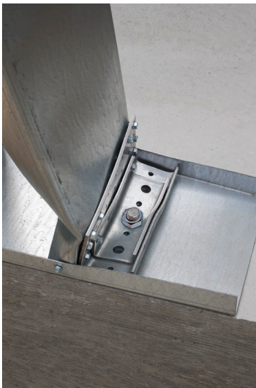
Assembly test with member failure
