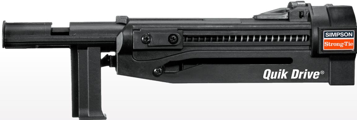
Use in conjunction with FHSD screws to drill through steel thicknesses 3-5 mm for mezzanine floor installations or the TBG screws to drill through 4-6 mm steel thicknesses for truck bed/trailer installations.
