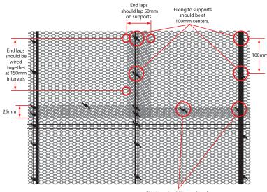
Side laps should be not less than 25mm and should be wired together at 150mm intervals. Fixing Expanded Metal Lathing to Solid Backgrounds
