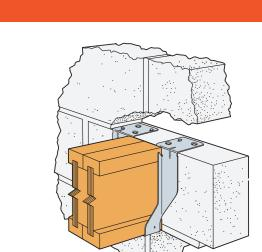
Heavy duty support for I-Joists from masonry walls.
