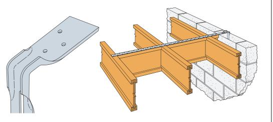
HES can be installed underneath the I-Joist top flange or placed above without the need for notching.
