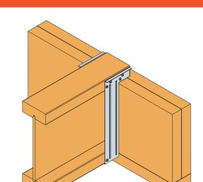
Install using CSA screws
