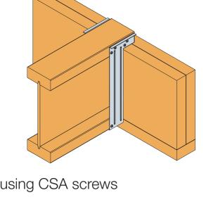
Top flange hanger available with skew or slope angles up to 45°.
