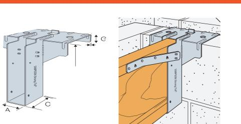
Face fix hanger for supporting I-Joists from timber members.
