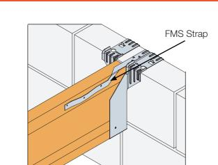
Supports I-Joists from masonry walls without the need for three courses of blockwork above.
