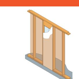
Provide racking resistance to timber frame structures with large openings. **Steel Strong-Portal**
