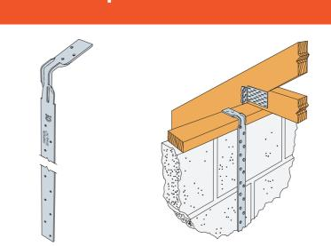
Vertical restraint for connecting wall plates to masonry walls.
