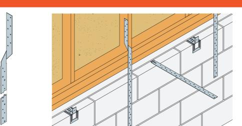
Restraint strap with a formed twist for timber to timber and timber to masonry connectors. Suitable for use in providing lateral / vertical restraint for timber gable panels.
