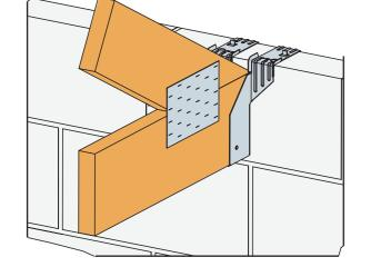
Supports trusses from masonry walls without masonry above the top flange.
