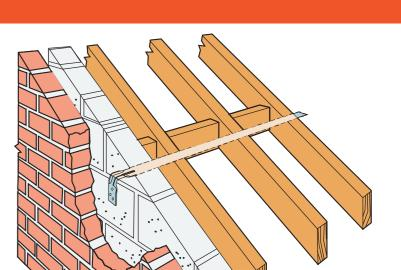
Connects trusses to gable walls. Just 1.5mm thick, the HES fits without notching.
