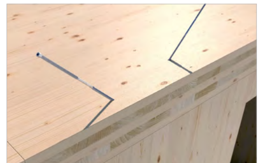
SWD inclined installation of CLT floor panels.
