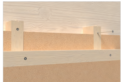
TTUFS screws in light wall framing.
