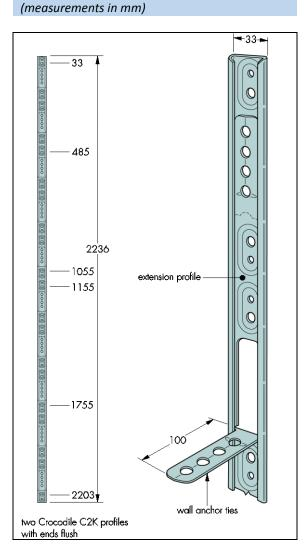
Figure 1 Crocodile C2K Wall Extension Profiles
