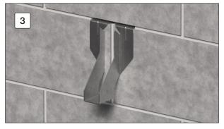
Insert the masonry hangers top flange into the cut slot, ensuring the top of the hanger sits flat on the supporting masonry and the hangers back flange is tight against the face of the masonry.
