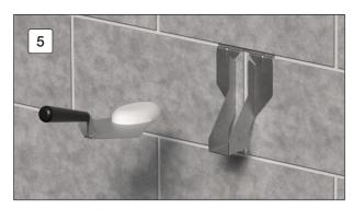
Force mortar or suitable epoxy resin into the slot and then allow to cure before applying load onto the hanger.
