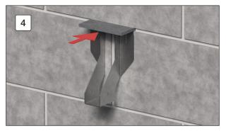
Tightly pack the void above the top of the hanger with an incompressible material (ie: slate) ensuring the full width of the hanger top flange is covered and the material is pushed all the way to the back of the slot, leaving the front 10mm of the slot clear.
