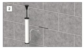
Brush and blow out all the dust and debris from the horizontal slot (ie: using a dust pump).
