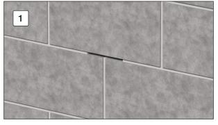
Cut out full height of mortar joist, at a depth and width enough to accommodate the top flange of the hanger.
