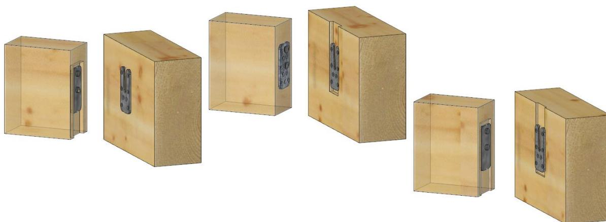
The connection to the header can be made with nails in the case where the header is prevented from rotation. In other cases, the CSA screws have to be installed.
